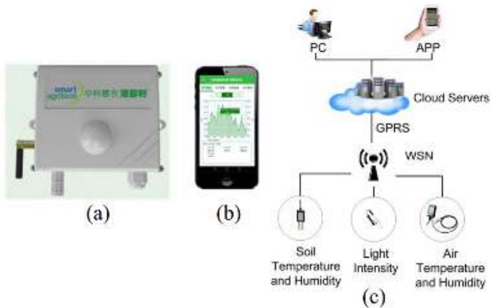
Figure 5.12 : IoT-based Pennellii-I environmental monitoring system. (a) Device, (b) App, and (c) system structure.
